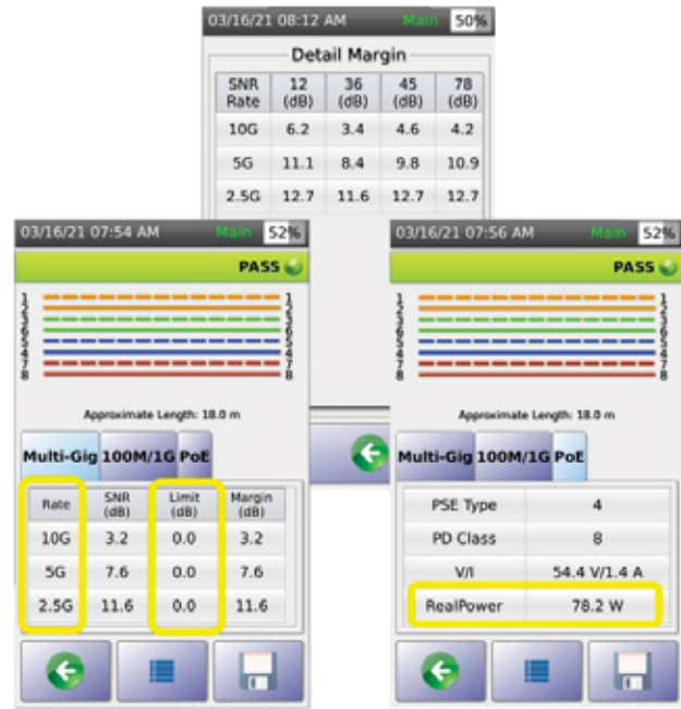
SNR based Multi-gigabit link speed testing while under both traffic and PoE
